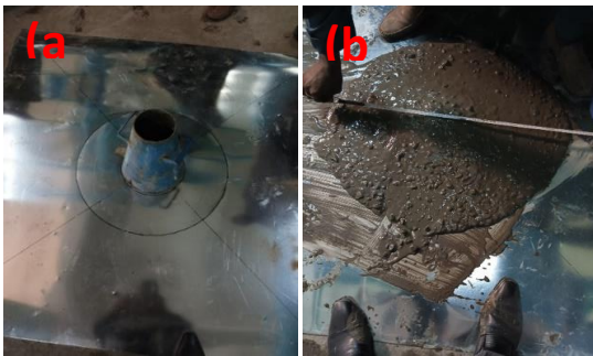
Figure 3 Slump Flow and T500mm Test (a. Slump Flow Apparatus, b. Slump Flow test)
